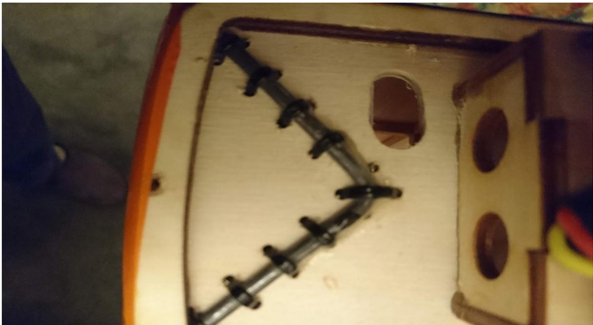
Undercarriage fixing to F1 showing 3mm cable ties
