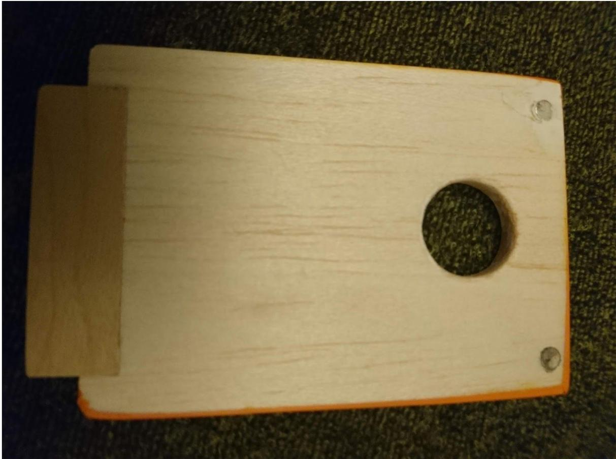
Inside of the hatch cover showing finger hole, magnets and ply locating tongue
