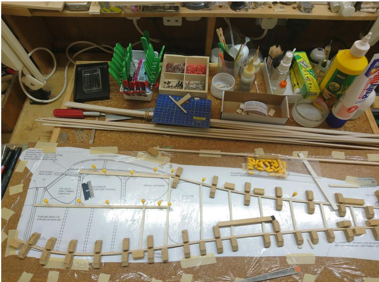
First fuselage side laid out after soaking longerons in water / ammonia bath.
