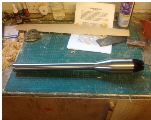
Pulse jet on work bench
